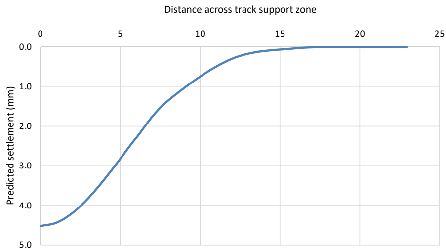
Figure 11 – Outputs from settlement calculations – worst case differential settlement across track support zone for railway crossing
